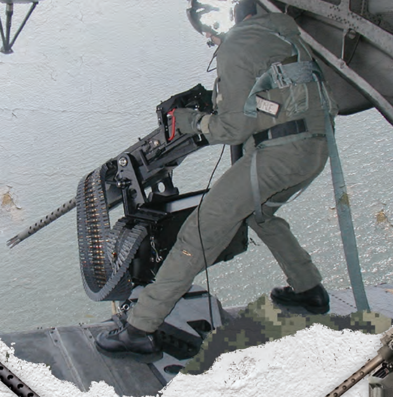
FN MEDIUM DOOR PINTLE WITH FN GAU-21 MOUNTED
